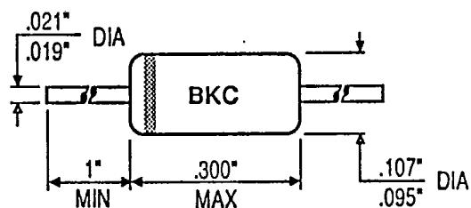
Passes all mechanical and environmental requirements of MIL-S-19500, including shock and vibration.
